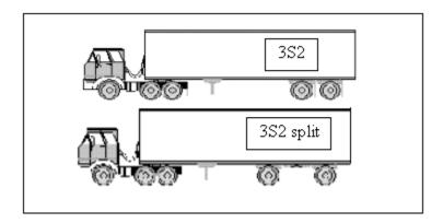
(LSIORB Class – Large Truck) FHWA Class 9 — 5 Axles, Single Trailer
