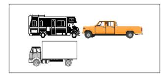
(LSIORB Class – Medium Truck) FHWA Class 5 — 2D - 2 Axles, 6-Tire Single Units (Includes Handicapped-Equipped Bus and Mini School Bus)
