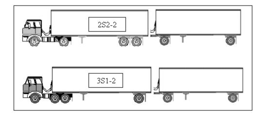
(LSIORB Class – Large Truck) Figure 1-25. FHWA Class 12 — 6 Axles, Multi-Trailers
